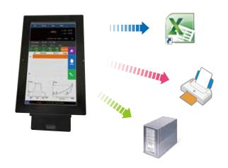
In addition to operation of a testing machine, Windows10 PC realizes many functions, such as data processing, printing, and connection with a network.
